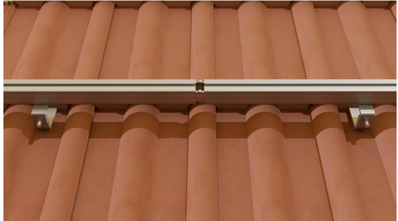
The graphic shows an example of the slide-in connectors including noses, which are hammered into the profile channel for a stable fit. Both mounting rails are pushed together flush on the connectors using pressure to create a positive fit.
